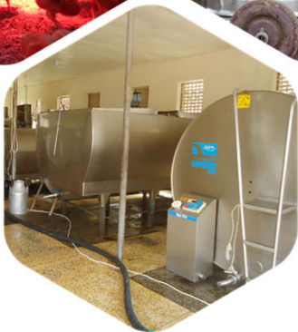
Solar bulk milk chiller
