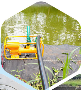
Solar water pump (SWP)
